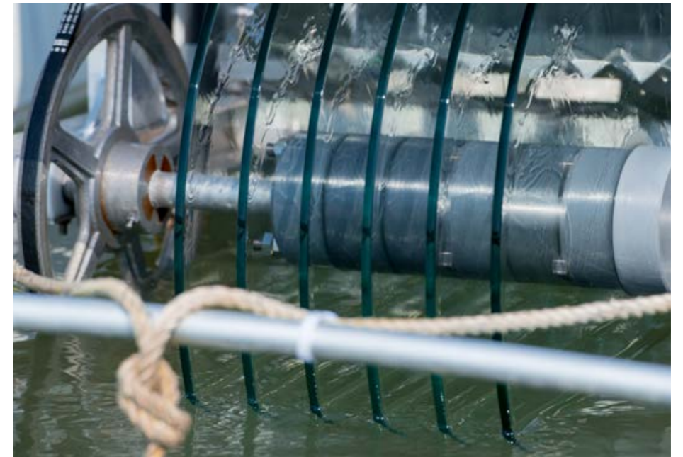
A sophisticated system: the rotating blades on the catamaran collect the surface film.
